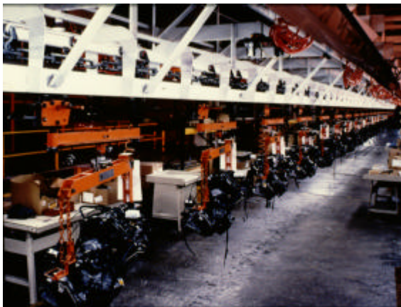
Figure 14.16. Power and Free Conveyor in Automotive Engine Assembly
