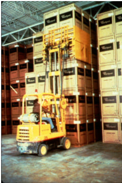
Figure 14.43. Block Stacking Household Appliances with Clamp Truck
