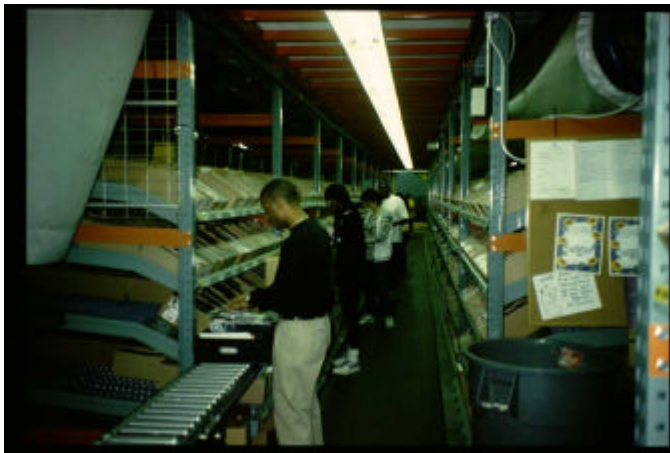
Figure 14.12. Roller Conveyor in Manual Order Picking (Photo courtesy of Dr. John Bartholdi)
