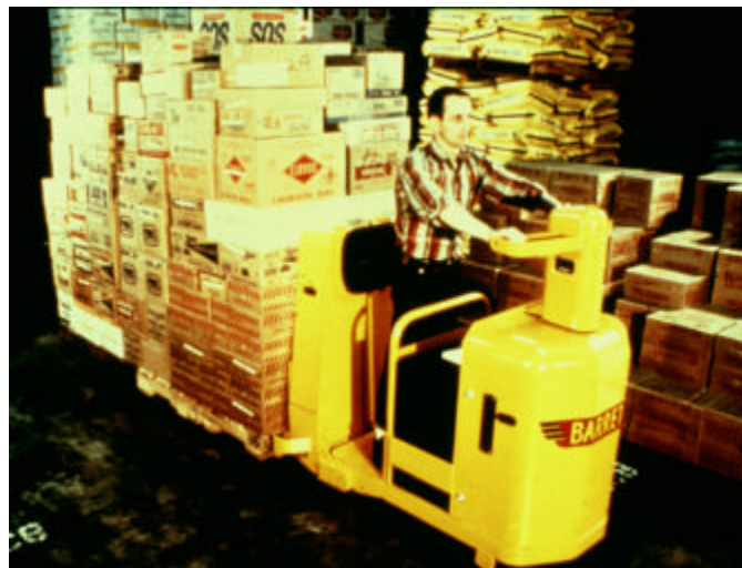
Figure 14.29. Tractor with Double Pallet Trailer Example
