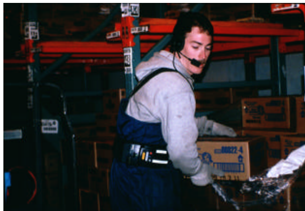
Figure 14.50. Radio-Frequency Communications during Order Picking in Cold Storage (Picture courtesy of Vocollect)
