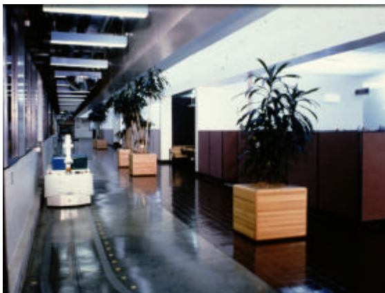
Figure 14.39. Multiload AGVS in Electronics Manufacturing
