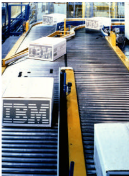
Figure 14.14. Roller Conveyor with Diverter in Electronics Manufacturing
