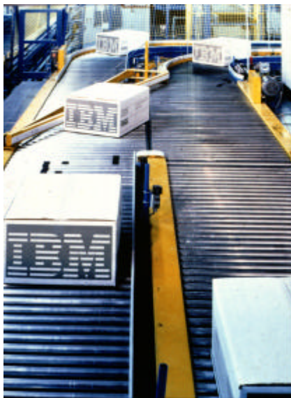
Figure 14.13. Roller Conveyor Network in Electronics Manufacturing
