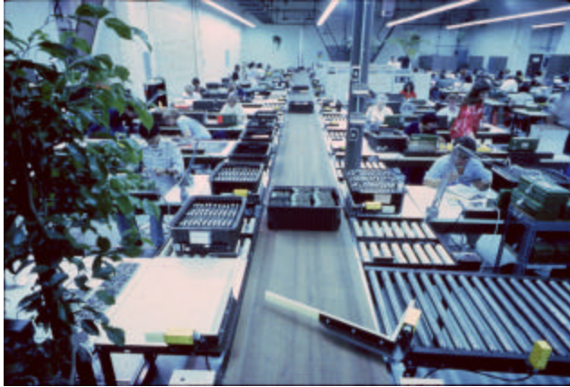
Figure 14.10. Belt Conveyor with Diverter Bar in Electronic Assembly
