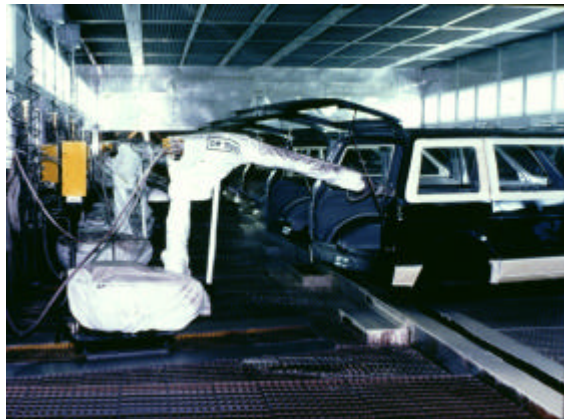
Figure 14.68. Robotic Spray Painting in Automotive Assembly
