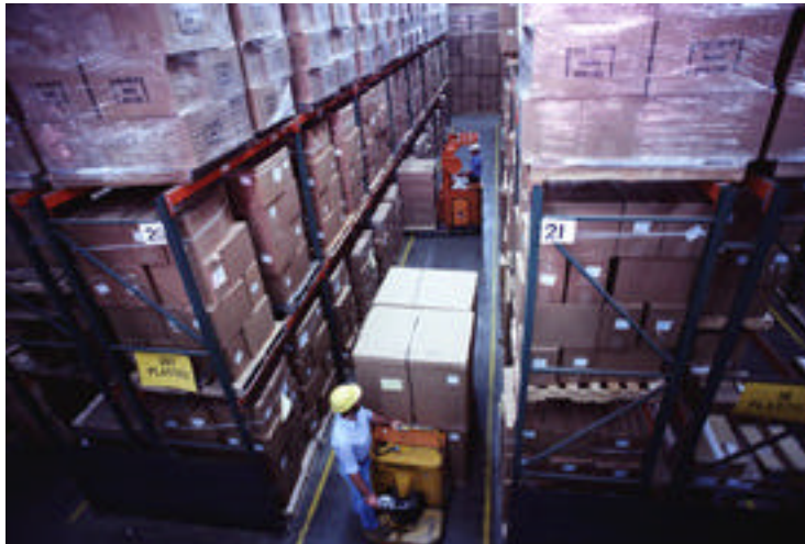
Figure 14.46. Unit Load Pallet Rack with Pallet Jack and Straddle Truck
