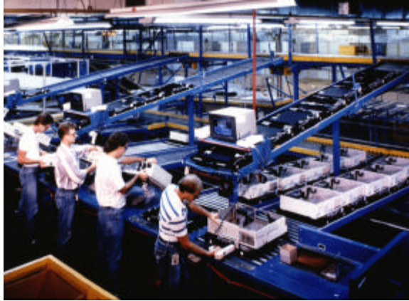
Figure 14.13. Roller Conveyor Network in Electronics Manufacturing
