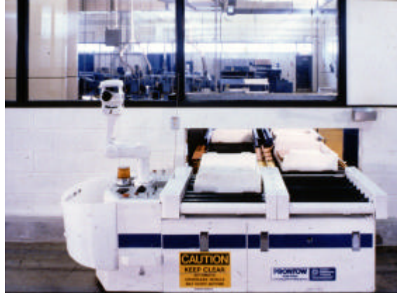
Figure 14.40. Multiload AGVS Interfacing with a Clean Room
