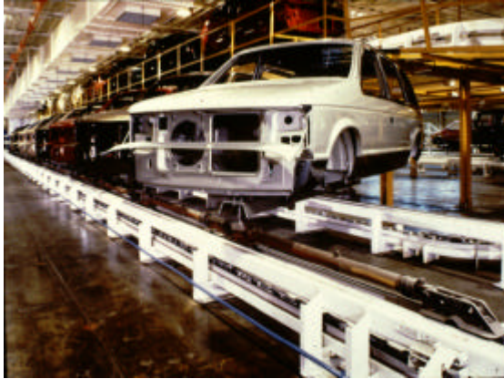
Figure 14.15. Inverted Power and Free Conveyor in Automotive Assembly
