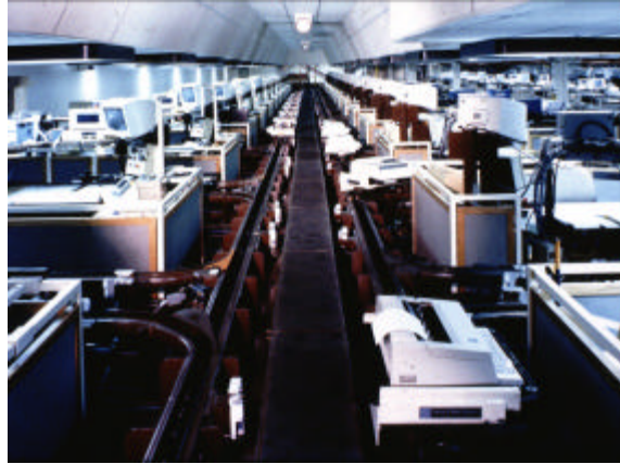
Figure 14.18. Inverted Automated Electrified Monorail in Typewriter Manufacturing
