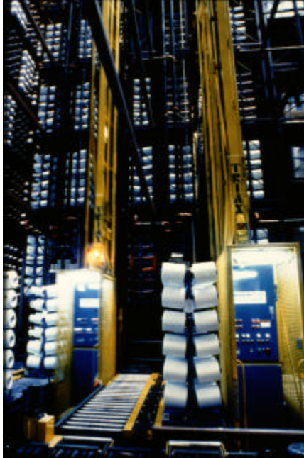
Figure 14.56. Unit Load Automated Storage/Retrieval System for Thread Coils
