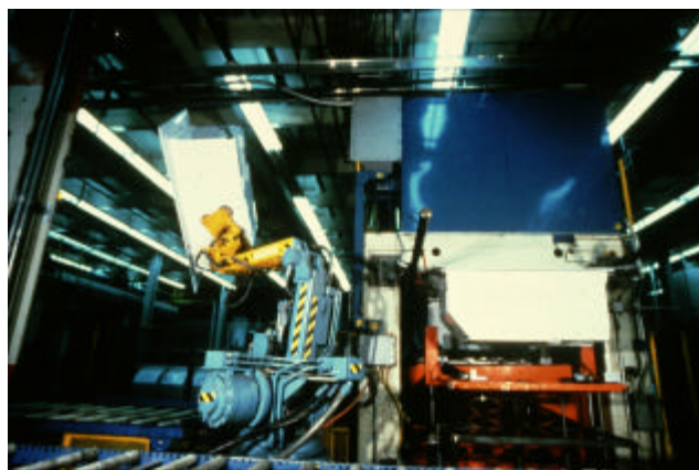
Figure 14.71. Robotic Part Unloading with Vacuum Gripper
