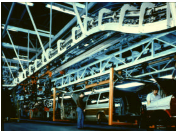
Figure 14.17. Power and Free Conveyor in Automotive Final Assembly
