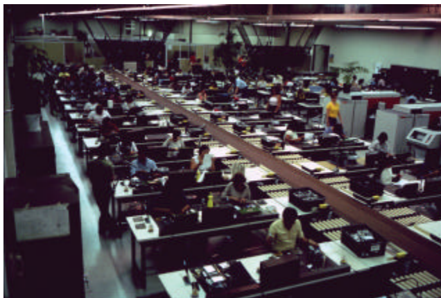
Figure 14.9. Belt Conveyor in Electronic Assembly
