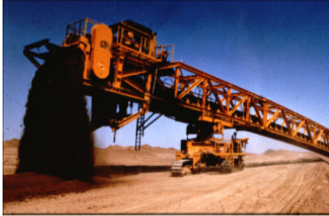
Figure 14.7. Bulk Belt Conveyor for Removal of Gold Mining Debris
