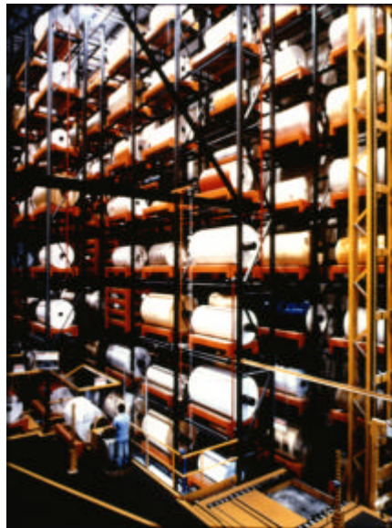
Figure 14.55. Unit Load Automated Storage/Retrieval System for Paper Rolls
