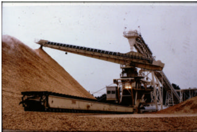
Figure 14.8. Bulk Belt Conveyor for Removal of Wood Chips
